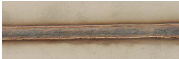
CrNi-Blech, 0,5 mm Kehlnaht am Überlappstoß, 1,0 mm CrNi-Draht
